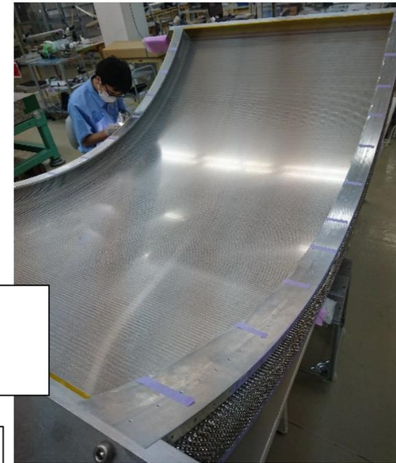
Resistive Plate Chamber:  $\Delta T \sim 60$  ps
