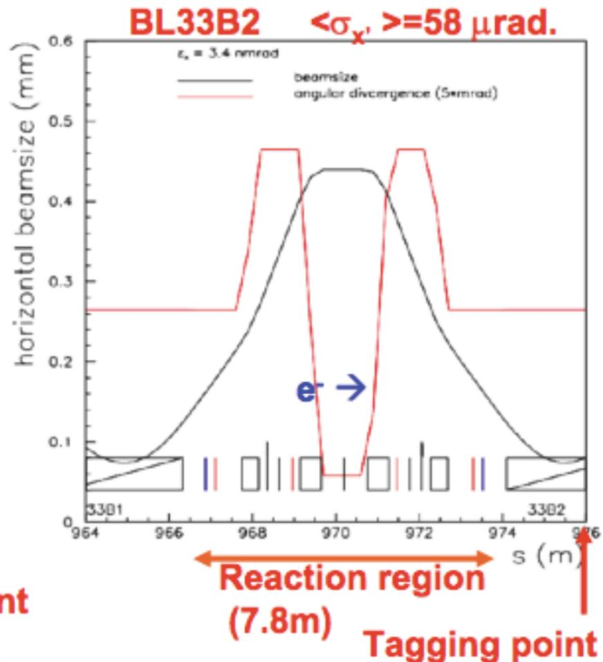
$\gamma$  rays are delivered to 150 m downstream.
