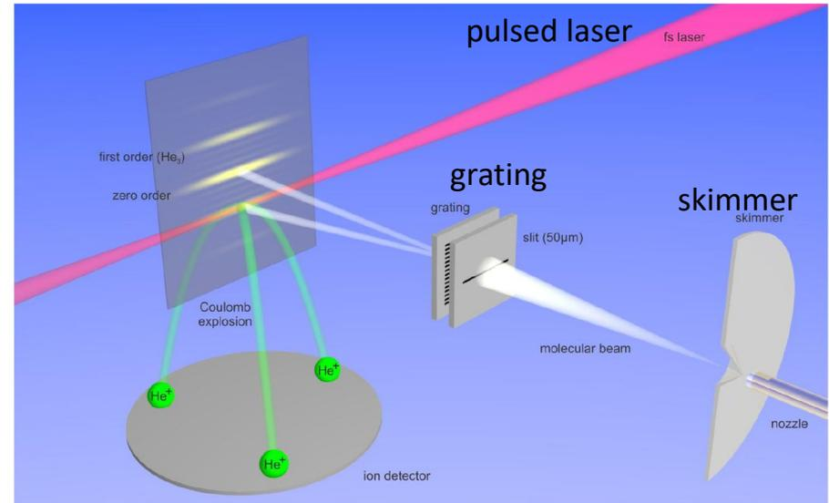
Efimov states are directly observed by ionization detection
