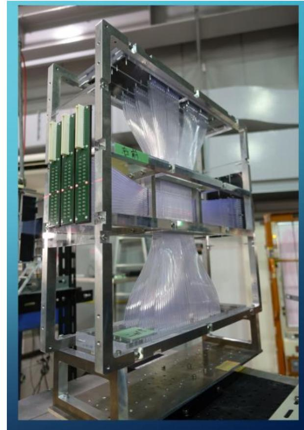
Active fiber target for energy loss correction
