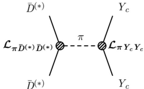
$$V^\pi(r) = -\frac{g_\pi g_1}{3f_\pi^2} \left[ \vec{S}_1 \cdot \vec{S}_2 C(r) + S_{S_1 S_2} T(r) \right]$$
