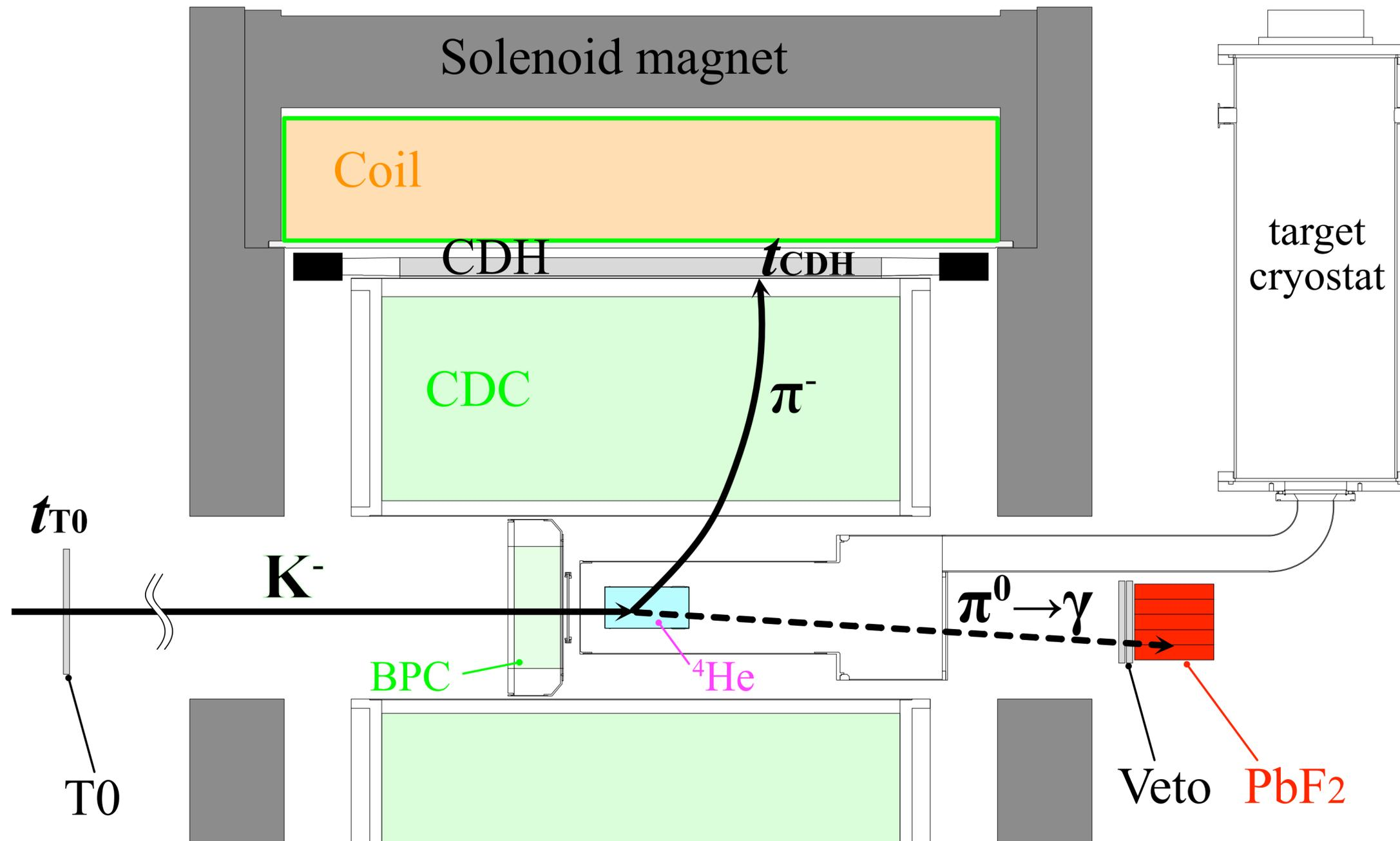
$$t_{\text{decay}} = (t_{\text{CDH}} - t_{\text{T0}}) - t_{\text{CDC}}^{\text{calc.}} - t_{\text{beam}}^{\text{calc.}}$$
