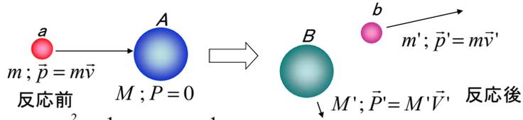
$$T = \frac{p^2}{2m} = \frac{1}{2} M_{tot} V_{CM}^2 + \frac{1}{2} \mu v_{rel}^2$$
