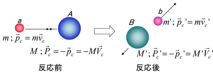
$$T_c = \frac{M}{m+M} T = \frac{1}{2} \mu v_{rel}^2 = \frac{1}{2} \mu' v_{rel}'^2 - Q$$
